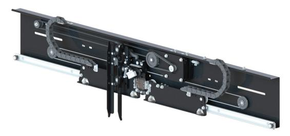
modern frequency regulated synchronous drive noise level <50 dB adjustable opening and closing speed power consumption in standby mode 4W up to 360 cycles per hour non-contact monitoring by a high-resolution light curtain EN81-20/50 conform
